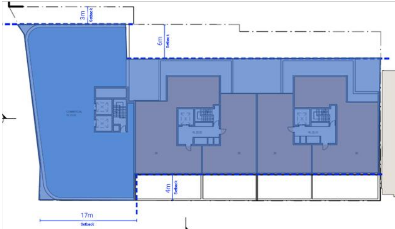
Figure 21: Proposed DCP setbacks at third floor level fronting New South Head Road and fourth floor level fronting Bay Street (Source: Tzannes)
